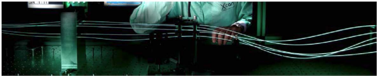
Fig. 1. Pictures of XCAN fluorescing Yb doped amplifying fiber
